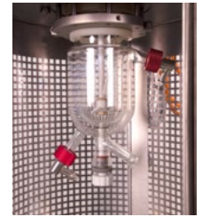
Glass vessel with Pt100-sensor and stirrer.
